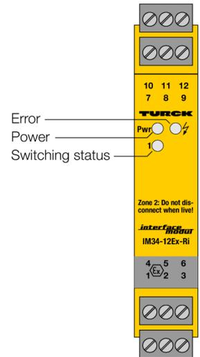
The 1-channel Ex-area temperature measuring amplifier IM34-12EX-RI is designed to evaluate the temperature-dependent changes of Ni100/Pt100 RTDs, thermocouples types B, E, J, K, L, N, R, S and T or low voltages in a range of -100...+160 mV and to output them as temperature-linear current signals 0/4...20 mA.
