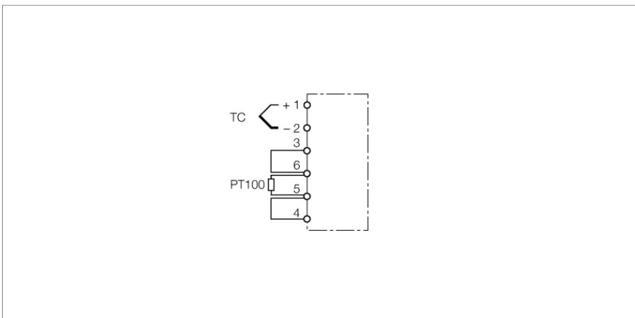
Temperature measurement with thermoelements requires a very precise determination of the reference point temperature. The IM-3-CJT offers this possibility.
