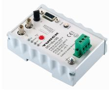
The optocoupler OC11Ex/3G.2 converts the PROFIBUS-DP signals into optical signals. The bus signals can therefore be transmitted from the safe area to the Ex area over long distances without potential or interference. When using fiber-optic cables, the maximum baud range is 2500 m for OM1 (62.5/125-µm) cables and 1500 m for OM2 (50/125-µm) cables.
