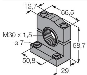
Mounting bracket, PBT black, for sensors with 30 mm thread, rotatable
