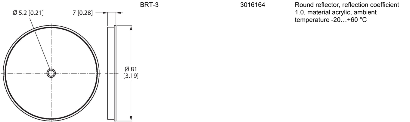
Dimension drawing Type ID
