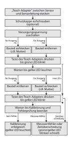
The measured signal in the sensor is influenced by the diameter and the material characteristics of the center bolt, but also by the cover of the sensitive area. Therefore, to ensure the correct switching behavior, each sensor must be conditioned to the operating environment, i.e. to the centering sleeve or closure cap used and the component to be detected (nut, sleeve, etc.). To configure a sensor, the teach adapter VB2-SP1 available from Turck is required.
