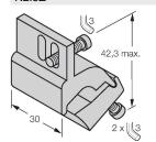
Mounting bracket for mounting magnetic field sensors on tie-rod cylinders; cylinder diameter: 32...63 mm; material: Aluminum
