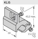
Mounting bracket for mounting magnetic field sensors on profile cylinders; cylinder diameter: 32...50 mm; material: Aluminum
