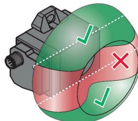
The left figure shows how the read/write head must be aligned towards the data carrier. As an example here the read/write head TNSLR-Q42TWD-H1147 is shown (instructions valid for all suitable read/write heads).
