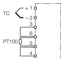
Temperature measurement with thermoelements requires a very precise determination of the reference point temperature. The IM-3-CJT offers this possibility.
