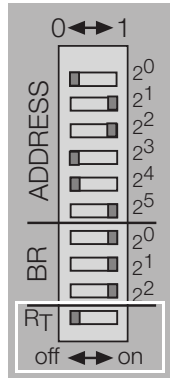
Fig. 9: Bus terminating resistor switched off
