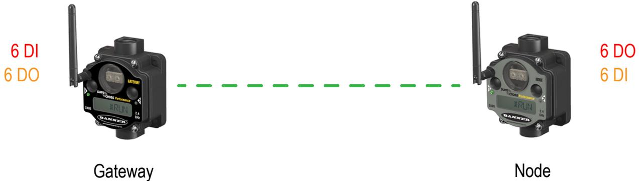
The SureCross® Performance Mapping kits create a radio frequency network with integrated I/O that can operate in most environments and eliminate the need for wiring runs. The Performance Mapping kits include one Gateway, which acts as the wireless network master device, and one Nodes. I/O mapping between the Gateway and Node are set using the Gateway's DIP switches.
