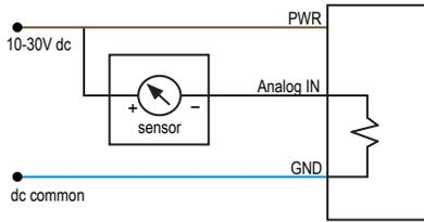
Analog Input Wiring (4–20 mA, 2-Wire, Externally-Powered Sensors)
