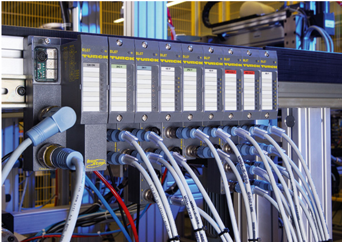
BL67 - up to 32 expansion modules can be added to the right of the gateway, without the requirement for a module rack or a mounting panel
