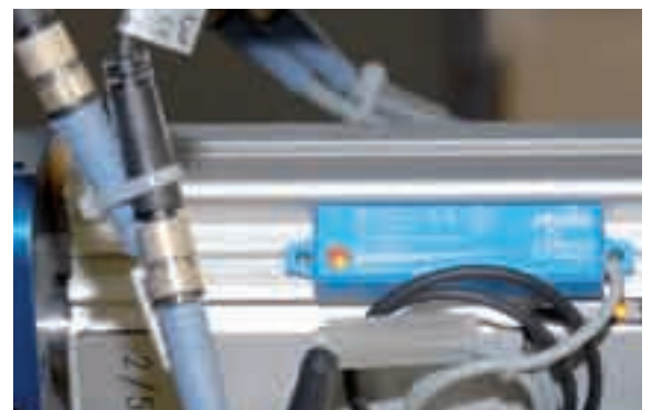
Turck produces analog magnet field sensors “FRIMO by Turck” especially for this application
